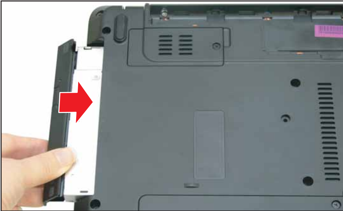
Figure 3:21. Installing the ODD Module
