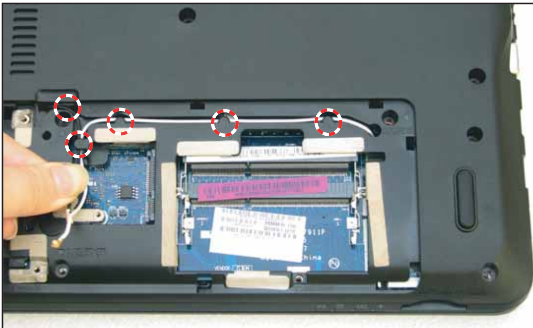
Figure 3:70. Routing the Antenna Cables (2 of 2)
