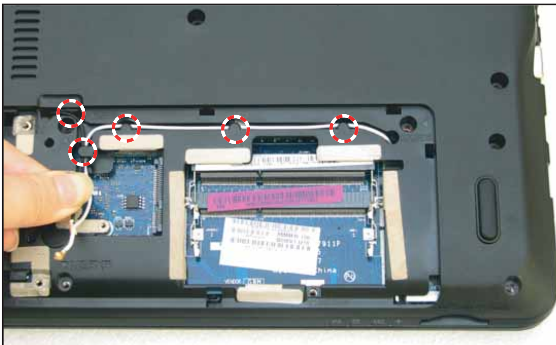
Figure 3:59. Removing the Antenna Cables (1 of 2)
