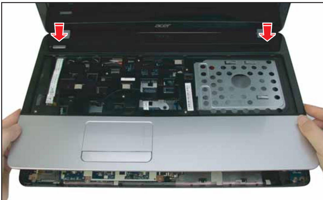
Figure 3:51. Installing the Upper Case (1 of 2)
