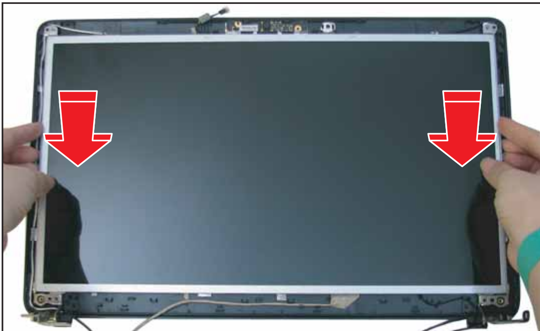
Figure 3:147. Installing the LCD Panel
