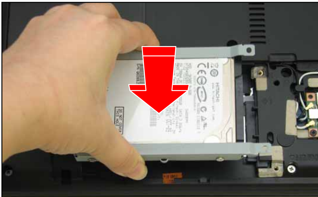
Figure 3:29. Installing the HDD Module (1 of 2)
