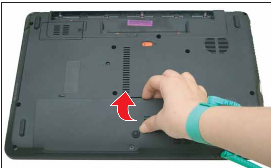
Figure 3:11. Installing the Base Door
