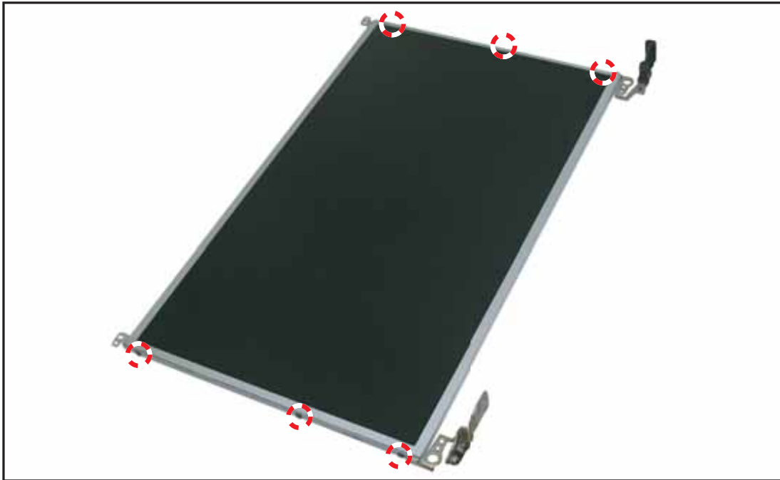
Figure 3:152. Installing the LCD Panel Brackets
