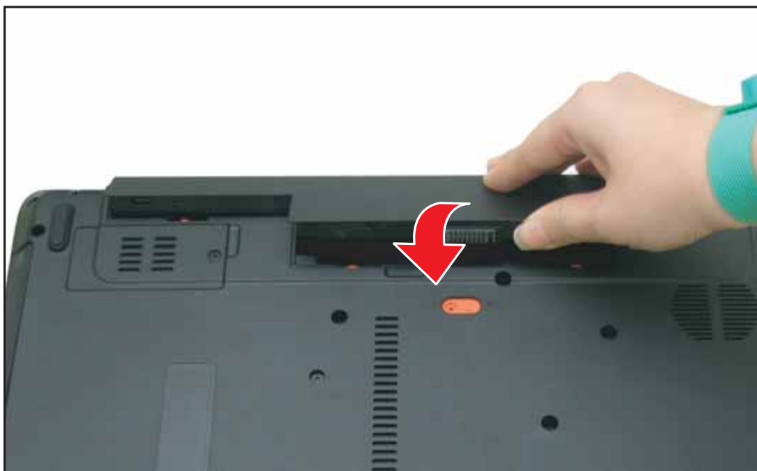
Figure 3:5. Installing the Battery Pack
