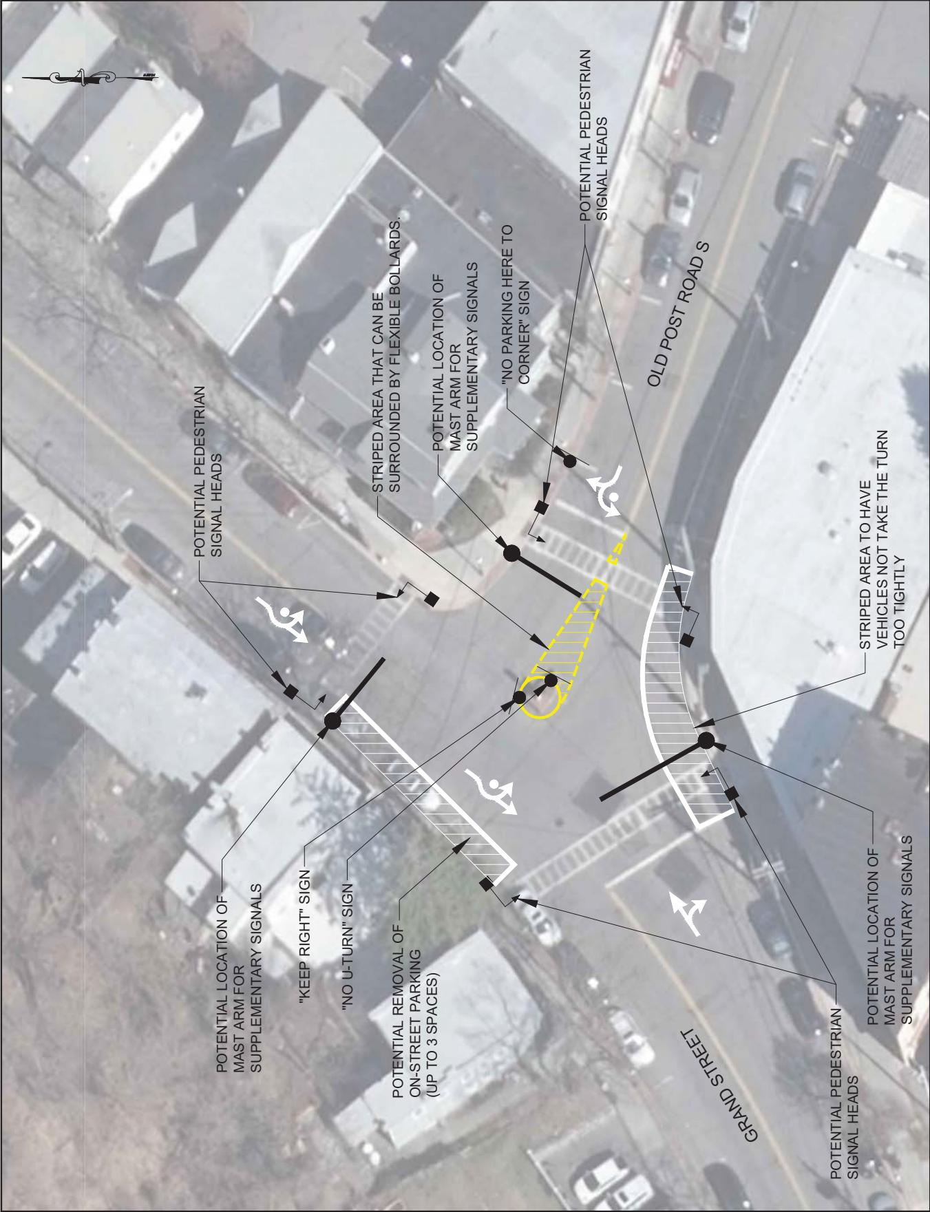
**CONCEPT PLAN 2A – REMOVAL OF “DUMMY” SIGNAL**
