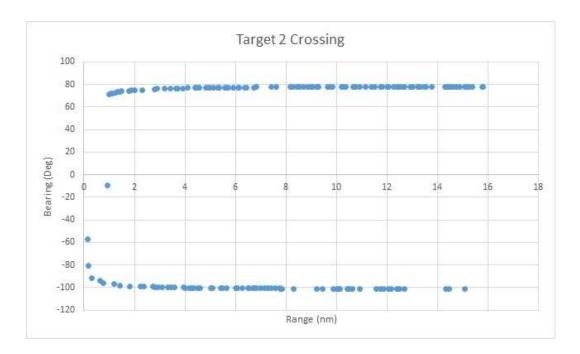
The above plots show how signal reception is affected as the target aircraft passes over Own Ship.
