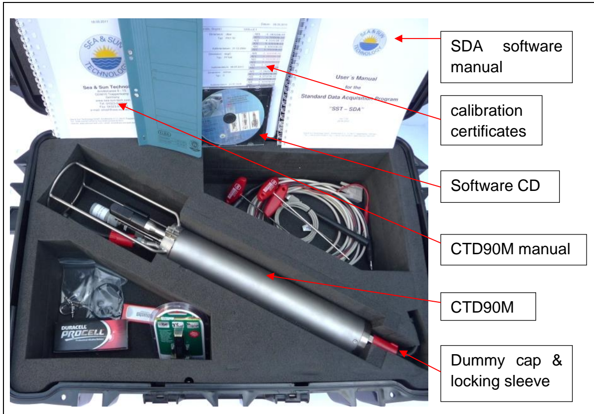
Figure 3: If there is no big frame as mounting device, the CTD90M is packed in a plastic suitcase.
