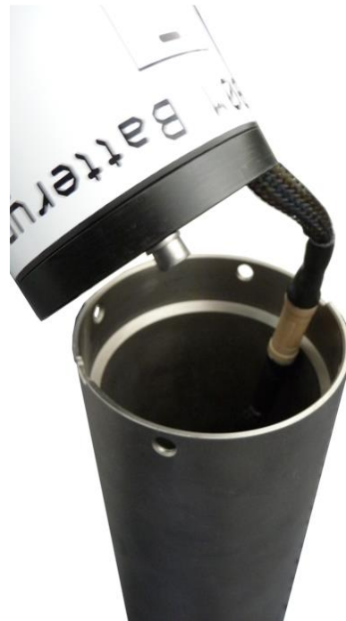
Figure 60: View inside the top end cap.
