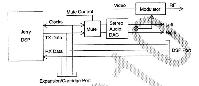
The Jaguar console includes a stereo 16 bit audio subsystem Digital audio data can only be sourced from the Jerry DSP. This data can also be monitored at the expansion or DSP ports, on the TXD serial data line. Jerry can also read serial digital audio data on its RXD pin. The bit clock and word strobe signals can be sourced by Jerry, the expansion port or the DSP port. If the clock source is not Jerry, then software must force the Jerry clock lines tristate, by clearing bit 0 of SMODE.
