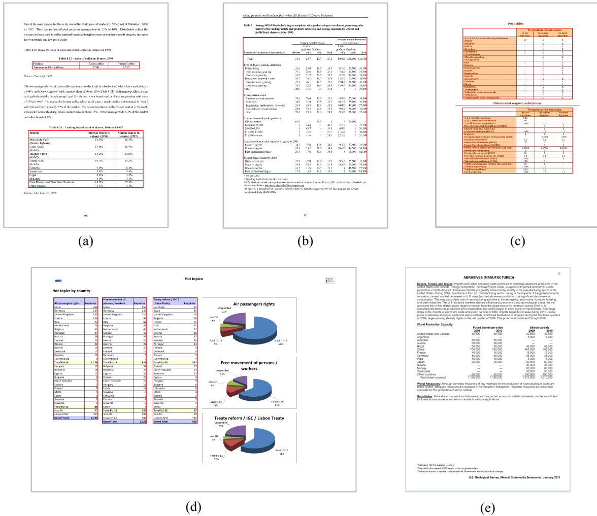
Fig. 6. Examples of proposed method, the table detection are marked by red rectangle.
