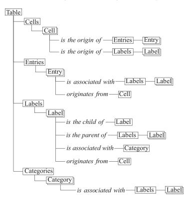
Figure 2: Two-layered table object model.
