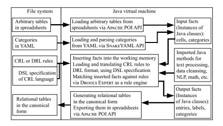
Figure 7: Architecture of TABBYXL, the tool for spreadsheet data canonicalization.
