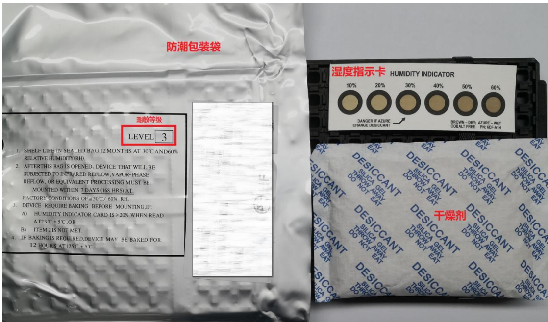
picture4-2Schematic diagram of dry vacuum packaging materials
