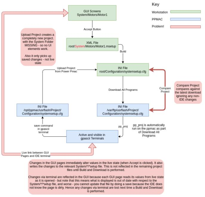
When you use the Add Motor context menu a new MotorX.msetup file is created. I assume that at this point all values are read from the current live state. This implies it is possible to re-create the GUI XML files from current state but that at present there is only a manual way of doing so.
