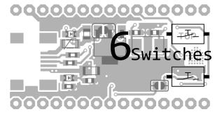
Put solder on the pads first, then place the switch and heat the pins from the top.
