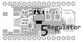
5V operation: close solder jumper. 3.3V operation: leave it open. Self-powered: Omit regulator. If you don't know what this all means, you want 5V;)
