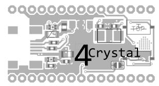
Put some solder on both pads. Place crystal on solder. Heat solder, gently pushing crystal.
