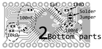
For the solder jumper, heat both pads and add lots of solder until they connect.
