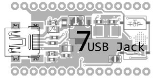
Solder the pins first. Check the solder joints. Then solder down the shield.
