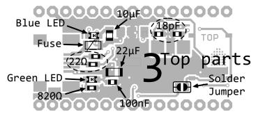
Start with the parts at the left and continue to the right. LED cathodes are marked.
