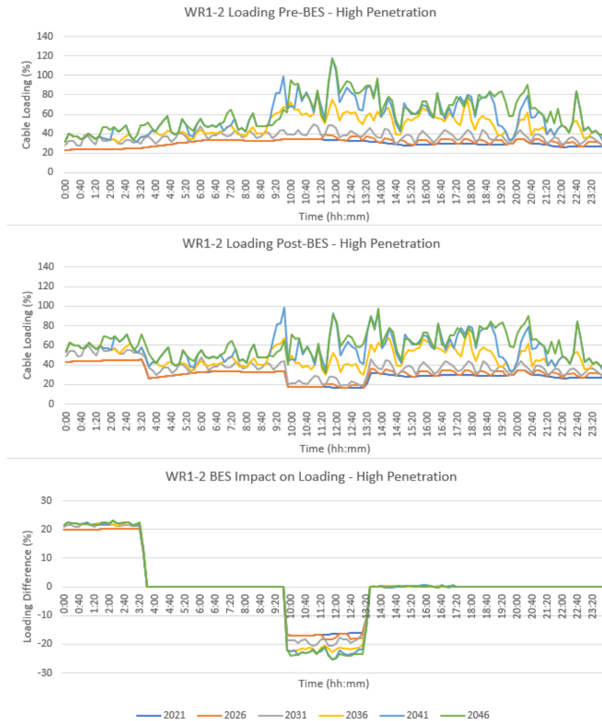
Figure 15: BESS impact on WR1-2 loading for high penetration scenarios. The top plot shows the hosting base case loading for WR1-2. The middle plot shows the loading on WR1-2 with the BESS included. The BESS loading impact is shown in the bottom plot.
