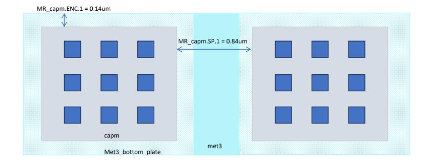
The space between CAPM is set by MR\_capm.SP.1. Met3\_bot\_plate (MR\_capm.SP.2) rule does not apply.
