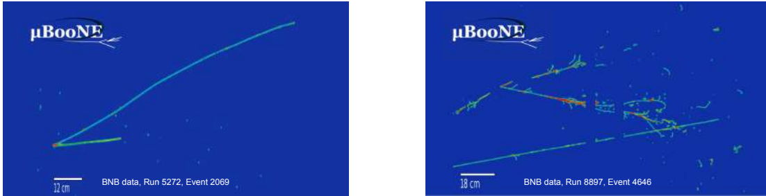
Figure 7.1: Examples of raw images of a neutrino interaction in MicroBooNE as recorded on the collection plane. The deposited charge (color scale) is shown as a function of wire number (x-axis) and time (y-axis). Left: Example of a \nu_{\mu}CC interaction with two tracks in the final state, identified as one proton and one muon. Right: Neutrino interaction containing three electromagnetic showers, which are identified as one electron and two photons, compatible with the signature of a \nu_e CC \pi^0 event.
