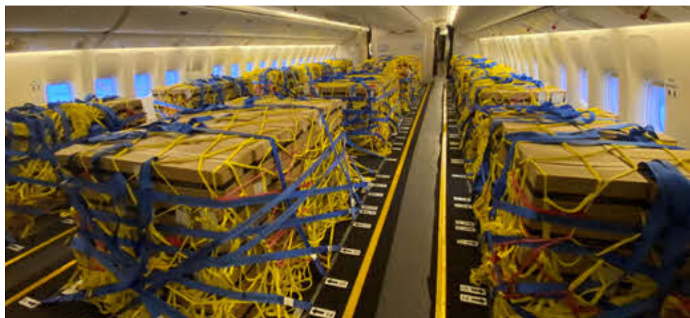
Seats were removed from the cabins of the Boeing 777-300ER passenger aircraft to increase its cargo capacity during the height of the pandemic.
