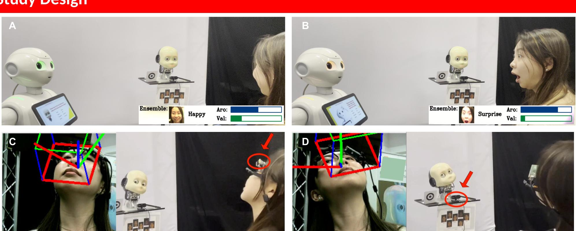
Experimental set-up within different conditions: A) The iCub mirroring facial expressions; B) The Pepper affectively signaling through LED color changes; C) The iCub mirroring head movement based on IMU readings. The red circle shows the IMU; D) The iCub mirroring head movement based on a vision-based model. The red circle shows the camera.
