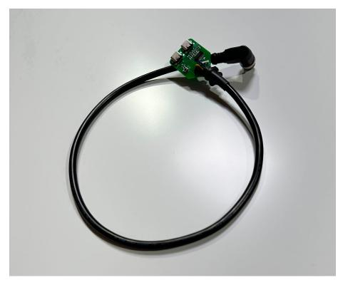
The Debug Cable is used to update and debug farm-ng products. It includes reset functionality along with USB and serial communication.
