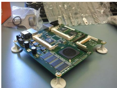
Affix the brackets to the board
