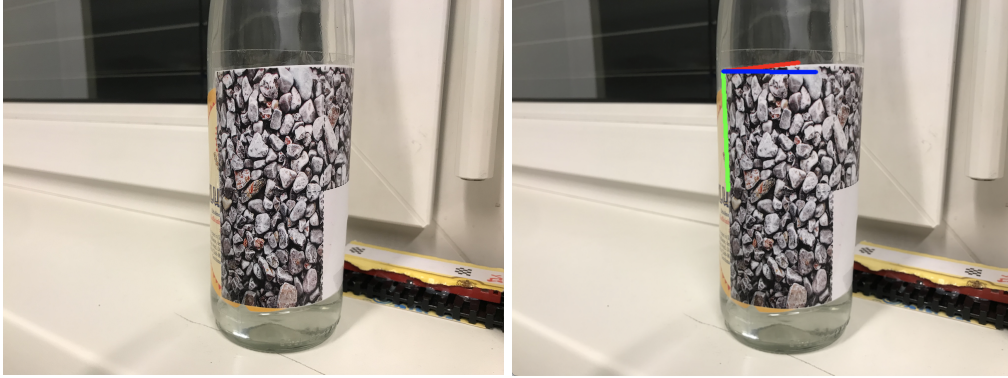
Figure 2: The printed reference image has been attached to a cylindrical object (bottle). (right) The axes of the reference are rendered onto the image.
