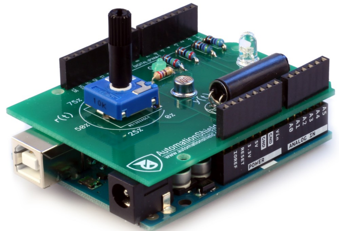
Fig. 1. The OptoShield control systems engineering educational aid mounted to an Arduino Uno.
