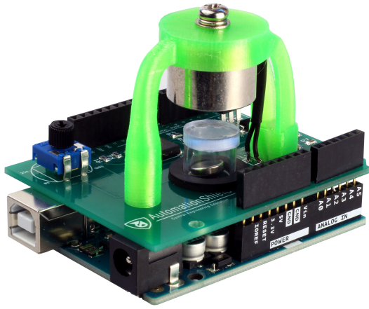
Fig. 1. Low-cost magnetic levitation experimental device prototype.
