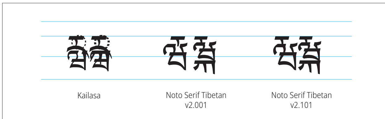
Fig 7. Kailasa.ttf broken substitution and Noto Serif Tibetan bug fix for Ra attachment.
