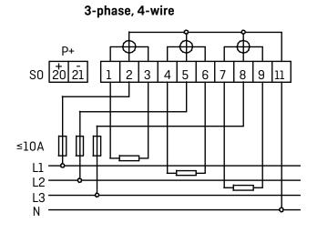
The valid connection diagram appears from the type label on the front of the meter.
