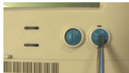
Figure 11: Release of sealable pushbutton.
