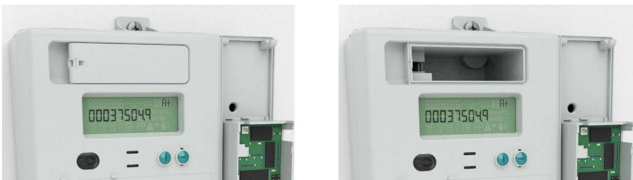
Figure 17: CCC-module area in OMNIPOWER.
