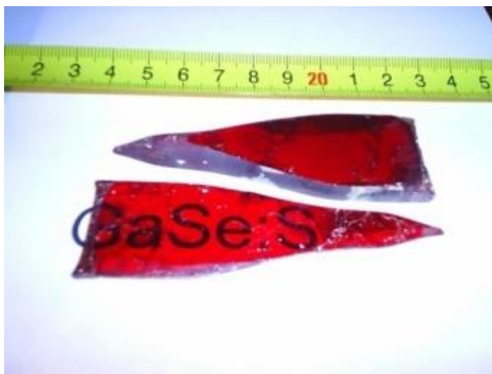
Figure. 1 Especially un doped and S doped (0.15 mass %) GaSe crystals grown by the Bridgman method.
