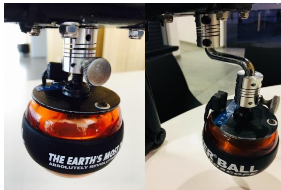
Fig. 9 - Direct and indirect coupling of the ball to the device.
