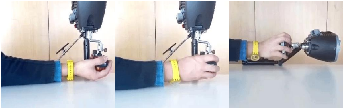
Fig. 8 - Different adjustments of the support and grabbing positions for different rehabilitation movements (from left to right: adduction/abduction, flexion/extension and pronation/supination).
