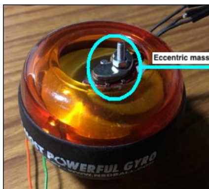
Fig. 5 - Eccentric mass that causes vibration to the ball on the device.
