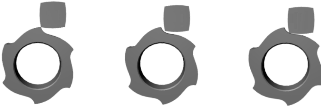
Fig. 4 - Illustration of the contact loss between the follower and the cam.
