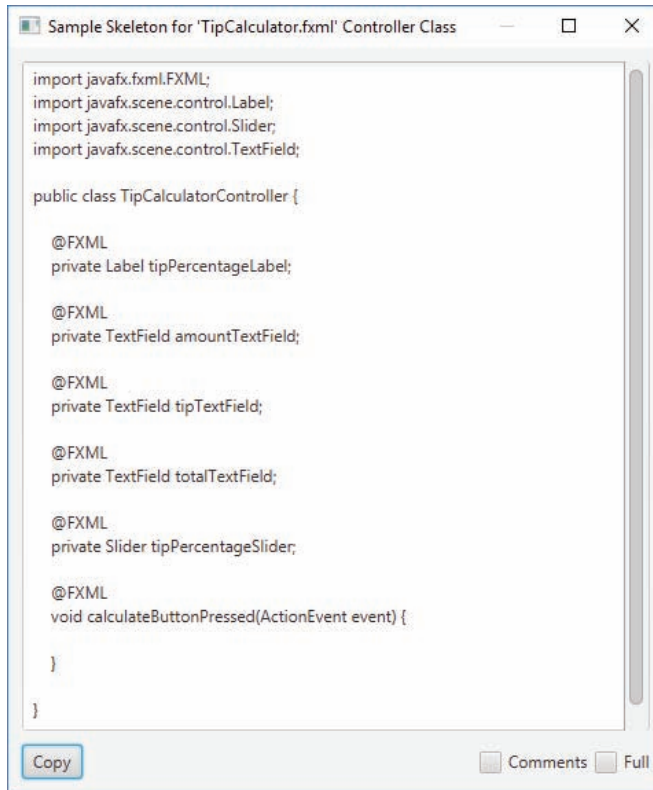
Fig. 12.18 | Skeleton code generated by Scene Builder.
