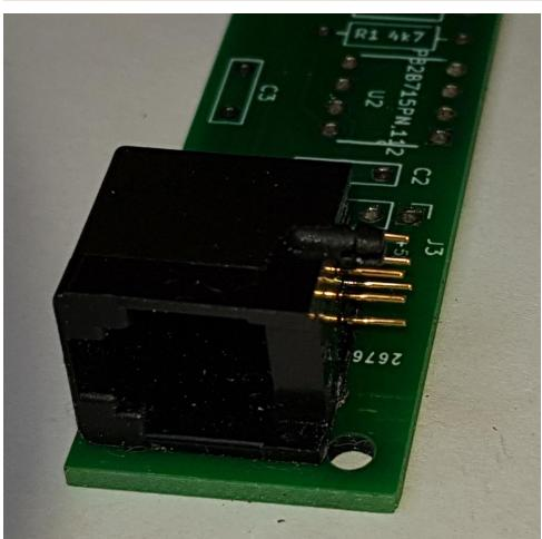
3. Now solder the connections with short wires (use silicon cable) from the board to the RJ11/12 connector like this:
