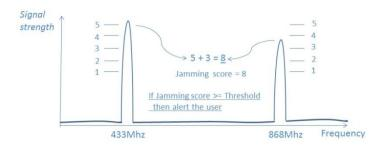
Note that with this principle, a threshold between 1 and 5 detects a disturbance on a single frequency, while a threshold between 6 and 10 requires disturbances on both frequencies, which threshold will dramatically reduce false positives. Of course, do not disable RECEIVER 433Mhz and/or 868Mhz when these receivers check jamming. Reception Frequency on each band is not important because jammers are dirty generators and do not transmit on precise frequencies.
