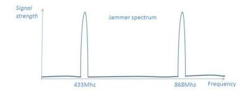
The RFPLAYER controls both frequencies 433Mhz and 868Mhz. Each frequency receives a score between 0 and 5. Then, the 2 notes are added and the result is compared to a user-programmable threshold. If the result is greater than or equal to the threshold, the user is alerted.
