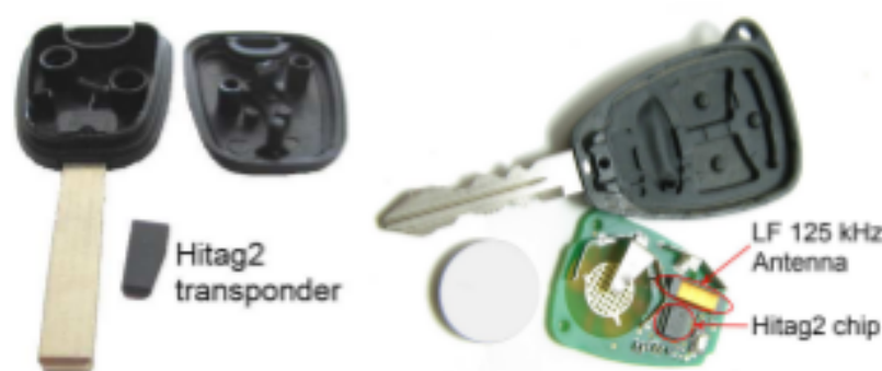
Figure 1: Car keys with a Hitag2 transponder/chip
