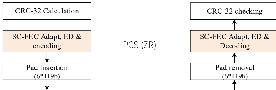
Figure 25: 400ZR HD-FEC processes
