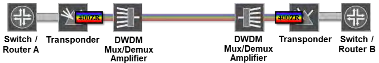
Figure 4: Transceiver line card with 400ZR DWDM interfaces
