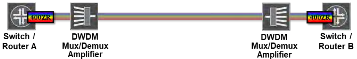
Figure 3: Router switch line card with 400ZR DWDM Interfaces
