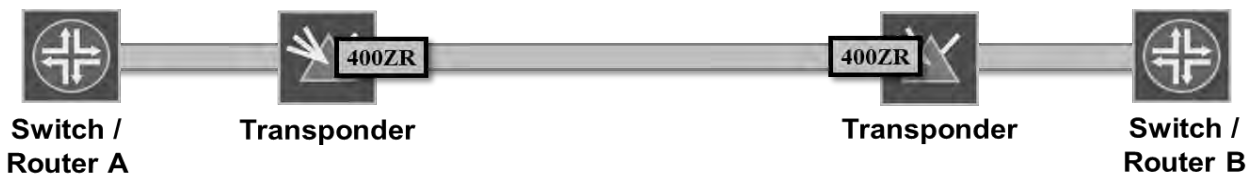
Figure 2: Transceiver line card with 400ZR amplified point-to-point interface
