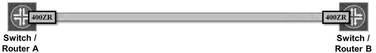
Figure 5: Router/Switch line card with 400ZR unamplified point-to-point Interface
