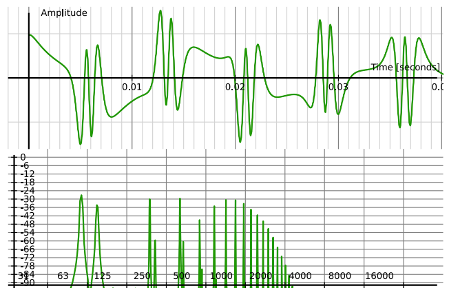
Figure 6: Exponential FM without DC correction.
