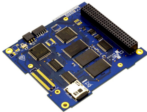
Figure 3. Example of OBC for CubeSats, the CubeComputer from CubeSpace. This model fulfill the CubeSat dimensions [27].
