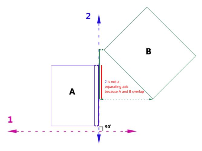
**Illustration:** The axis 2 is not a separating axis because A and B overlap, which implies there is no separating line parallel to axis 1.
