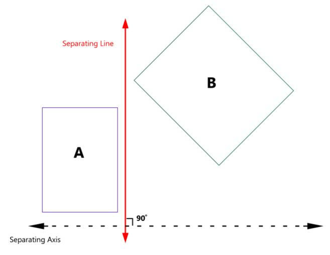
**Illustration:** Rectangle A and rectangle B are divided by a line, also known as a separating line. The separating line is perpendicular to the separating axis.
