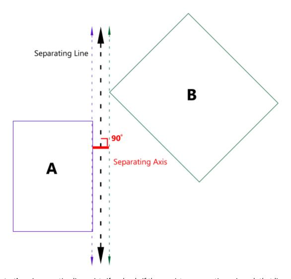
**Illustration:** A separating line exists if and only if there exists a separating axis such that lines may extend between polygons A and B.
