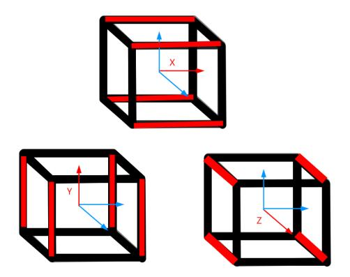
**Illustration:** The 12 edges of a box and their corresponding parallel axes. Notice for the topmost box, there are 4 edges parallel to the local x-axis of the box.
