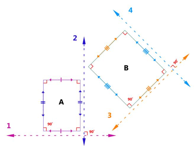
**Illustration:** Since separating lines exist only when there exists a separating axis that is coincidentally parallel to one of the edges, we need only consider the axes of the edges. This is because the edges of each rectangle are perpendicular to one another. Thus, we can use the axes of the edges to check whether there exists a separating axis.
