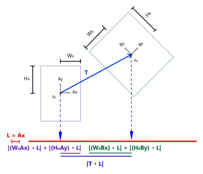
**Illustration:** The vector T and half of rectangles A and B are projected onto the axis L= Ax (or – Ax). The magnitudes of the projections are compared side by side at the bottom of this illustration. Notice, in this case,  $|T \cdot L| > |(W_A Ax) \cdot L| + |(H_A Ay) \cdot L| + |(W_B Bx) \cdot L| + |(H_B By) \cdot L|$ . Thus, L = Ax is a separating axis. However, notice that L = Ay and L = By are not separating axes for the case in this illustration.
