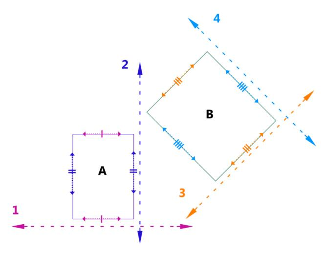
**Illustration:** To find whether rectangle A and B intersect, we need only consider 4 possible separating lines, which are parallel to the edges of rectangle A and B.
