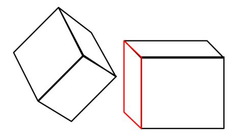
**Case Study 2:** Consider the two boxes in the illustration above. The two boxes are clearly not in collision, yet, there is no separating plane spanned by the axes of an edge from one box and an edge from the other box. However, the two boxes are not intersecting, so there must be a separating plane that separates them. A separating plane that separates the two boxes is parallel to a face (outlined in red) of one of the boxes.
