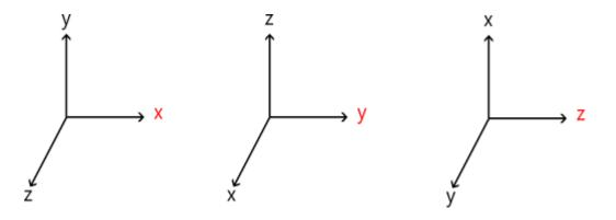
**Illustration:** We orient the XYZ coordinate system with respect to Y and Z to make their corresponding axes to the XYZ coordinate system with respect to X more apparent. Notice Y in the system with respect to X is equivalent to Z in the system with respect to Y.
