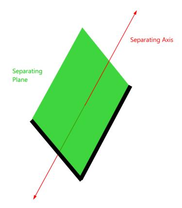
**Illustration:** The separating axis perpendicular to the separating plane can be found by taking the cross product of the axes of the two edges. The two edges are the black lines in the illustration.
