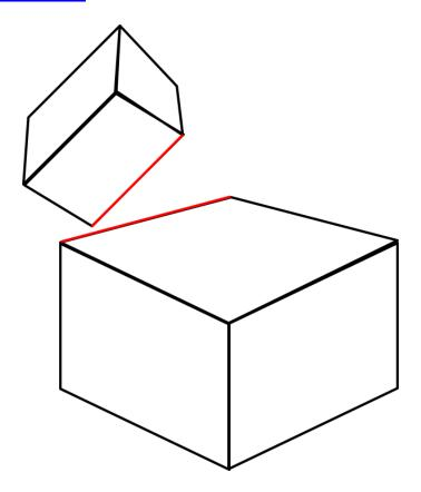
**Case Study 1:** Consider the two boxes illustrated above. The two boxes are clearly not intersecting, yet, there is no separating plane parallel to any of the faces. However, the two boxes are not intersecting, so there must be a separating plane that exists. A separating plane that separates the two boxes is spanned by the axes of the two edges (one from each box), highlighted in red.
