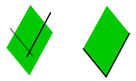
**Illustration:** In 3D space, the picture on the left depicts a green separating plane between the two edges. Since the plane exists and separates the two edges, it must be the case that the two edges do not intersect. The picture on the right depicts the separating plane parallel to the plane spanned by the axes of the two edges. Note: The separating plane spans infinitely and is not finite as depicted here in the illustration.
