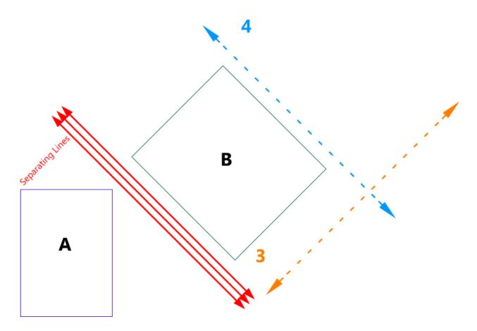
**Illustration:** There exists separating lines parallel to axis 4, but there is no separating line parallel to axis 3 that separates rectangles A and B.
