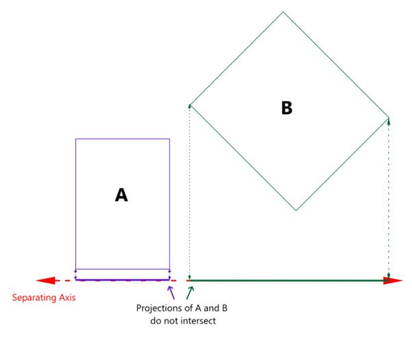
**Illustration:** Polygons A and B do not intersect because there exists a separating axis such that the projections of A and B onto the axis do not intersect.
