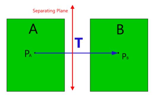
**Illustration:** Two 2D faces side-by-side lying in the same plane in 3D space. Clearly the two faces are not intersecting, but our approach in 3D space will interpret the two faces as intersecting. Notice, in this case, the only separating axes checked are perpendicular to both of the faces. Also, notice these separating axes checked cannot be depicted in the illustration above because they are going in and coming out of the page.
