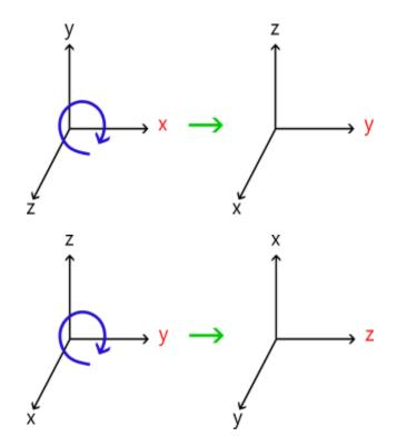
**Illustration:** 1) From X, we rotate the coordinate system to get the system with respect to Y. 2) From Y, we rotate the coordinate system to get the system with respect to Z.
