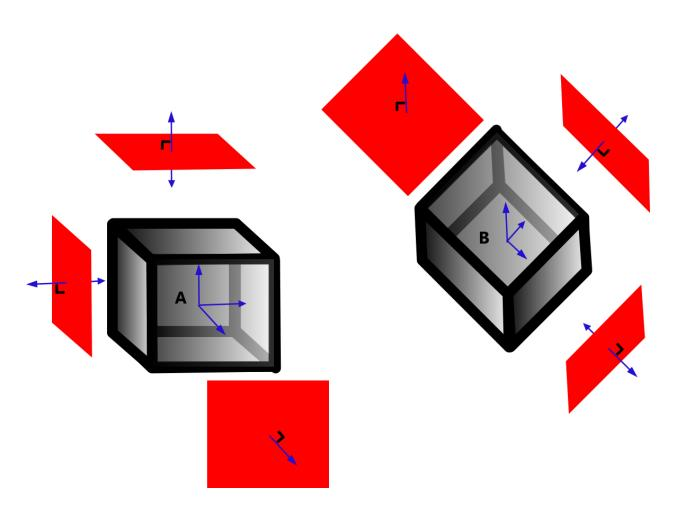
**Illustration:** The separating planes of interest are depicted in red, while the separating axes of interest are depicted as blue arrows intersecting the red planes. Notice the red separating planes of interest are parallel to the faces of the boxes. Also note the blue separating axes of interest are parallel to the local XYZ axes (also depicted in blue) of the boxes.
