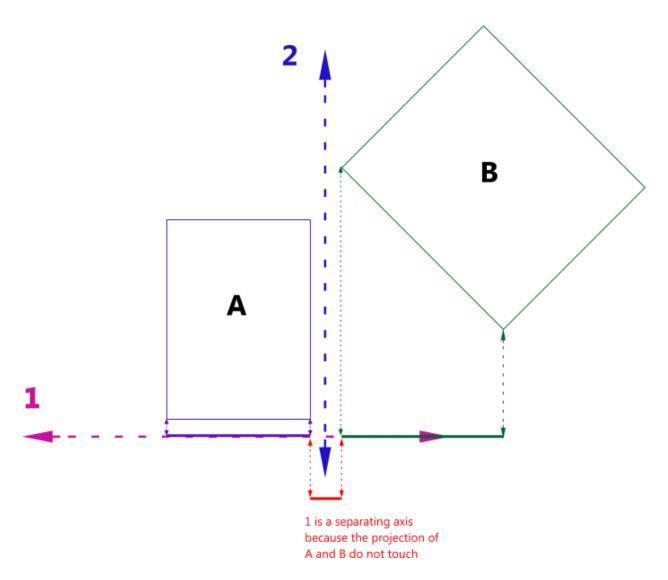
**Illustration:** The axis 1 is a separating axis because the projections of rectangles A and B onto axis 1 do not overlap nor touch one another, which implies there is a separating line parallel to axis 2.
