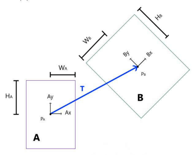
**Illustration:** T extends from the center of A to the center of B. This is why we only use half the dimensions of rectangle A and rectangle B.
