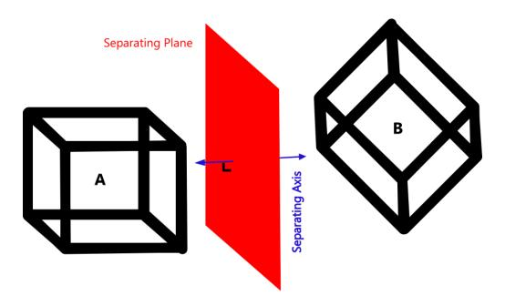
**Illustration:** The separating plane in 3D space contrasts with the separating line in 2D space. The separating plane separates box A from box B. In this particular illustration, the separating plane is parallel to the right and left faces of box A.
