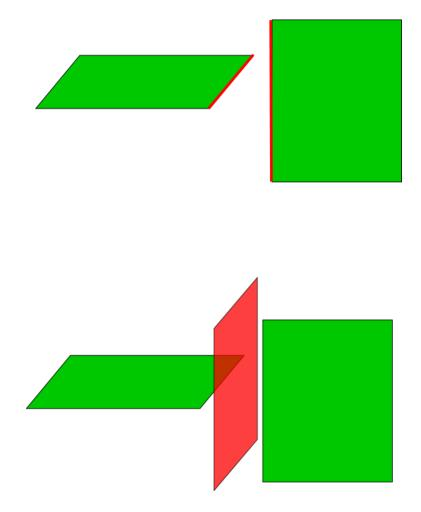
**Illustration:** The above image depicts two non-intersecting green faces. A separating plane that separates the two faces is spanned by the axes of the two edges highlighted in red. The bottom image depicts a separating plane.
