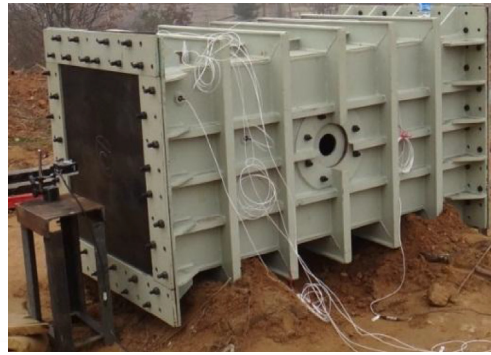
Fig. 1. Test facility of stiffened plates under confined blast load.
