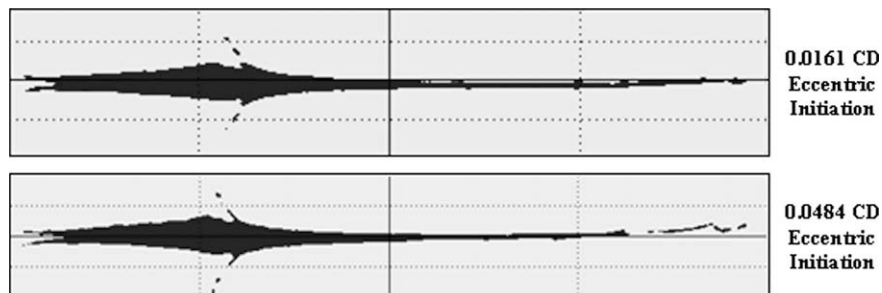
Fig. 6. Jets from eccentricity initiated shaped charges (50 \mu s from initiation).
