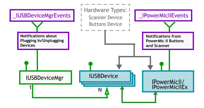
The **IUSBDeviceMgr** object manages events from all USB devices (including the *PowerMic II*) by providing a **DeviceCount** property to determine how many devices have been connected and a **Device** property to retrieve an object for the device.
