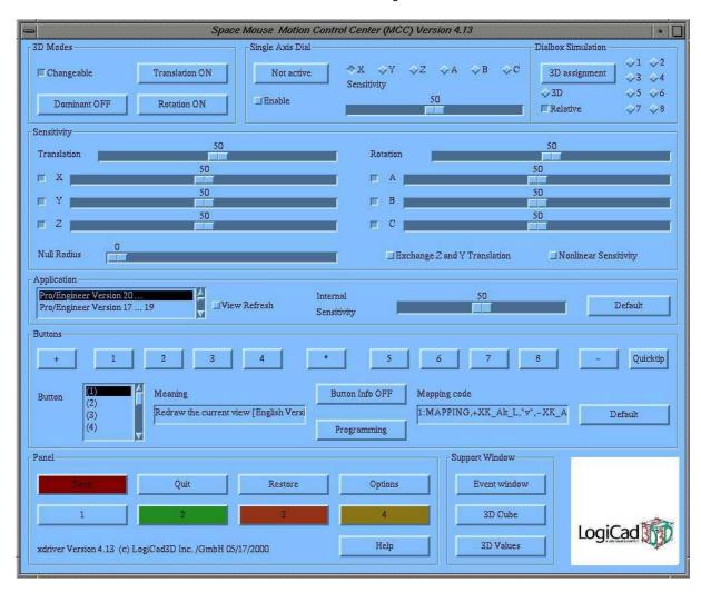
Null Radius [slider bar]. Controls the minimum displacement of the cap necessary to cause movement of the onscreen object. Increasing the null radius may be helpful in work environments prone to vibrations (e.g. industrial environments), which may cause the Magellan/SPACE MOUSE to register unintentional movements.
