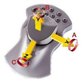
Note that the values input by Magellan/SPACE MOUSE are not interpreted as absolute position commands but as velocity commands. When the cap is displaced translationally or rotationally by a constant amount (a distance measurement), the graphical object is assigned a continuous speed in the same direction (a velocity measurement). The magnitude of the cap's displacement determines the magnitude of the onscreen object's velocity.
