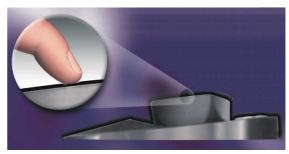
button that may be programmed just like the normal hardware buttons. The default function assigned to Quicktip toggles the driver window between the foreground and background. Note that for the Magellan/SPACE MOUSE Classic and Plus, the translation and rotation must be turned ON and the dominant mode turned OFF for the Quicktip function to work.
