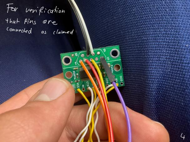
Geneval Setup with the Poluly Adaptor Connected to Pi as per Roadme
