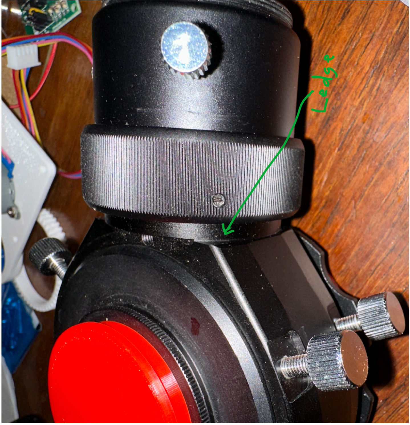
Note that there is a ledge that may provide some support to offset the thinner base section around the OAG tube.
