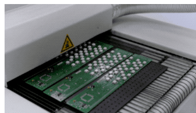
Figure 2: Circuit boards on oven belt (image licensed from Adobe)
