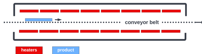
Figure 4: Reflow oven schematic diagram
