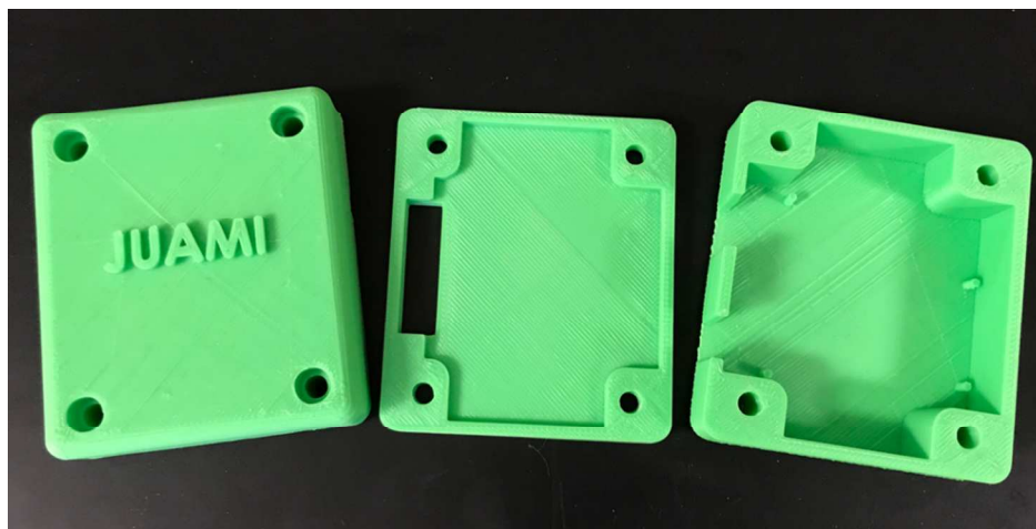
Figure S2. The 3D printed casing from the .stl files. From left to right are the top, middle and bottom pieces, which are assembled together with screws in the corners.
