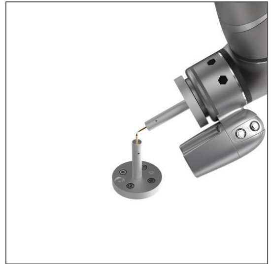
Figure 107: The Robot Posture Needs to Change during Teaching (1/2)
