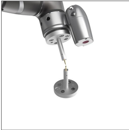
Figure 107: The Robot Posture Needs to Change during Teaching (1/2)
