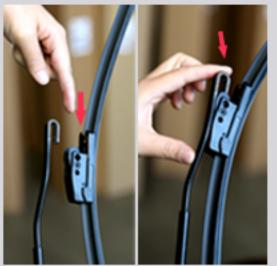
Step 2: Slide the new wiper blade over the J-hook as shown the pictures before.
