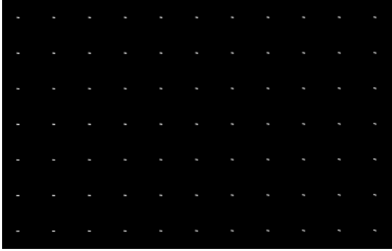
Figure 4. (Example 1) Spatially-varying blur kernels generated by scene motion in Figure 3
