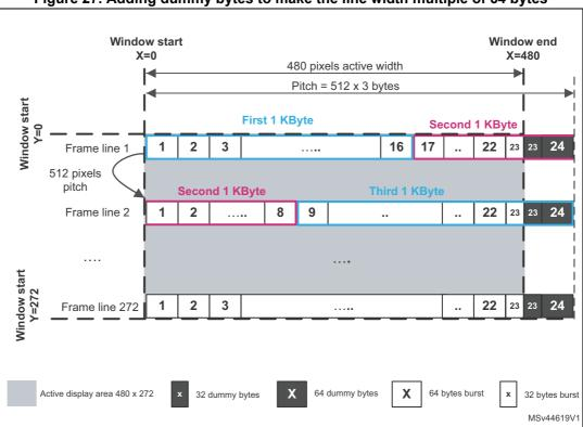
Figure 27. Adding dummy bytes to make the line width multiple of 64 bytes
