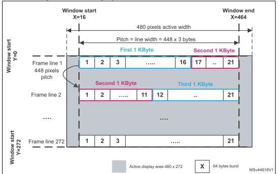
Figure 26. Reducing layer window and framebuffer line widths
