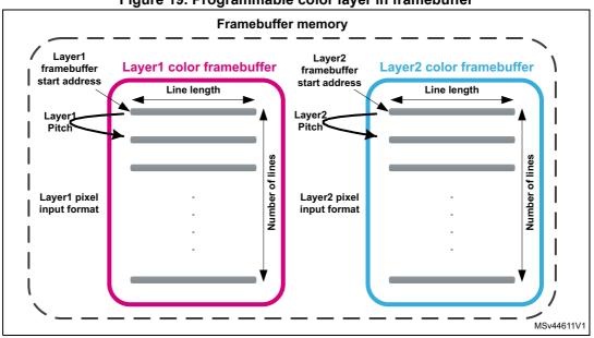
*Figure 19* summarizes all layer color framebuffer configurable parameters.
