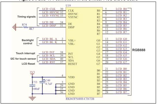
Figure 34. LCD-TFT connection in the STM32F746G-DISCO board
