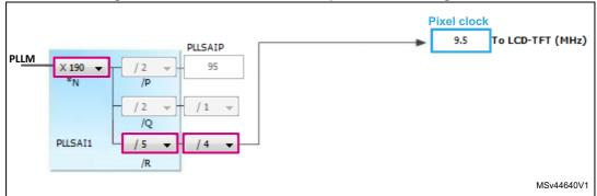
Figure 45. STM32CubeMX: LTDC pixel clock configuration
