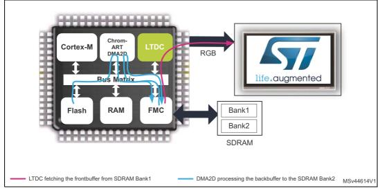
Figure 22. Typical graphic hardware configuration with external SDRAM
