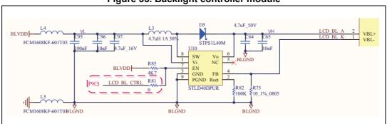
Figure 35. Backlight controller module
