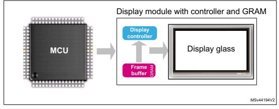
Figure 2. Display module with embedded controller and GRAM
