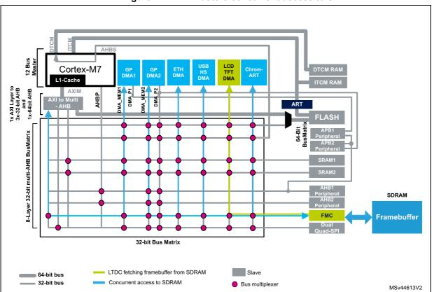
Figure 21. AHB masters concurrent access to SDRAM
