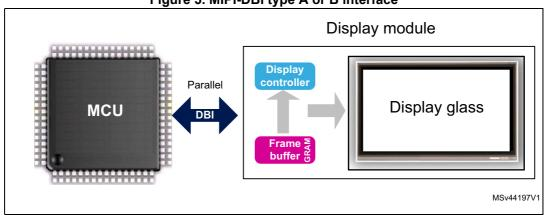
Figure 5. MIPI-DBI type A or B interface
