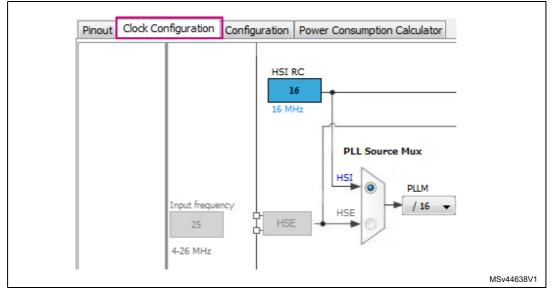
Figure 43. STM32CubeMX: clock configuration tab
