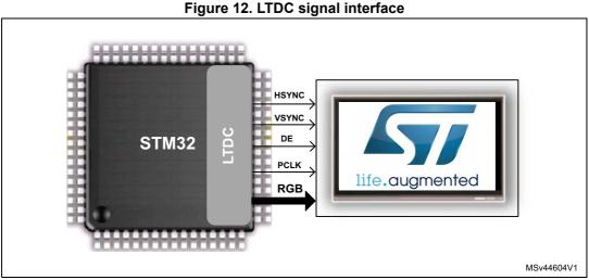
The LTDC can output data according to the following parallel formats: RGB565, RGB666 and RGB888. So a 16-bit RGB565, 18-bit RGB888 or a 24-bit RGB888 display can be connected.
