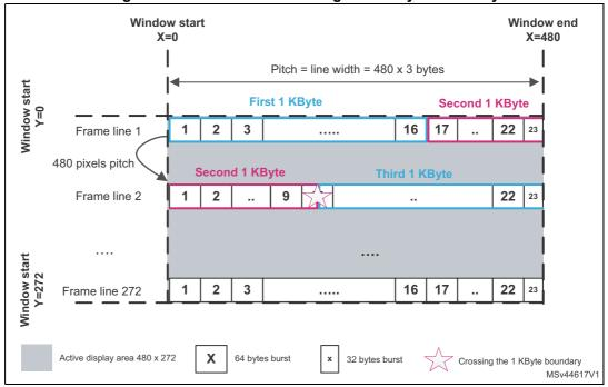
Figure 25. Burst access crossing the kilobyte boundary
