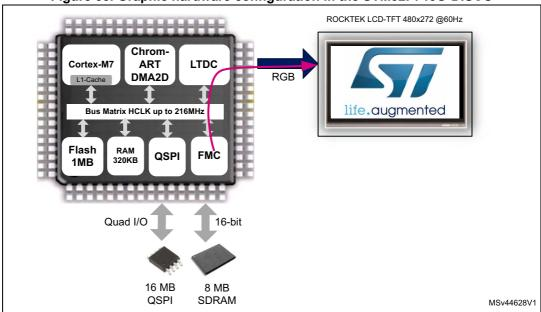
Figure 33. Graphic hardware configuration in the STM32F746G-DISCO
