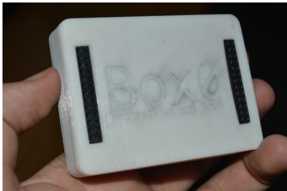
Figure: Box0 Enclosure, 3D printed
