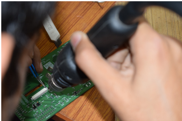
Figure: diy-VT100 rev3 soldering using hot air gun
