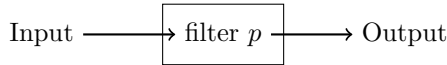
Figure 1.4: Input: [x_1, x_2, \dots, x_n] , Output: [x'_1, x'_2, \dots, x'_m] . and \forall x'_i \Rightarrow p(x'_i) .
