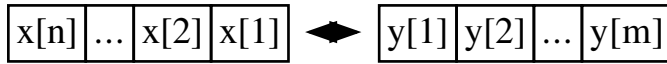
Figure 12.6: A paired-array list, which is consist of 2 arrays linking in head-head manner.
