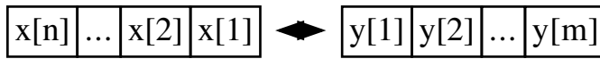
Figure 12.6: A paired-array list, which is consist of 2 arrays linking in head-head manner.
