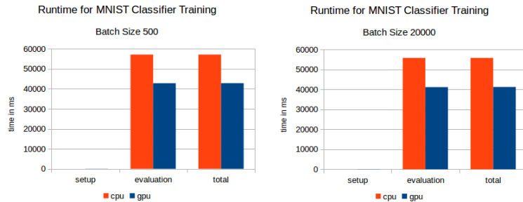
Fig. 12. Performance timings for 10 epochs of training the MNIST classifier for batch sizes of 500 (left) and 20000 (right).
