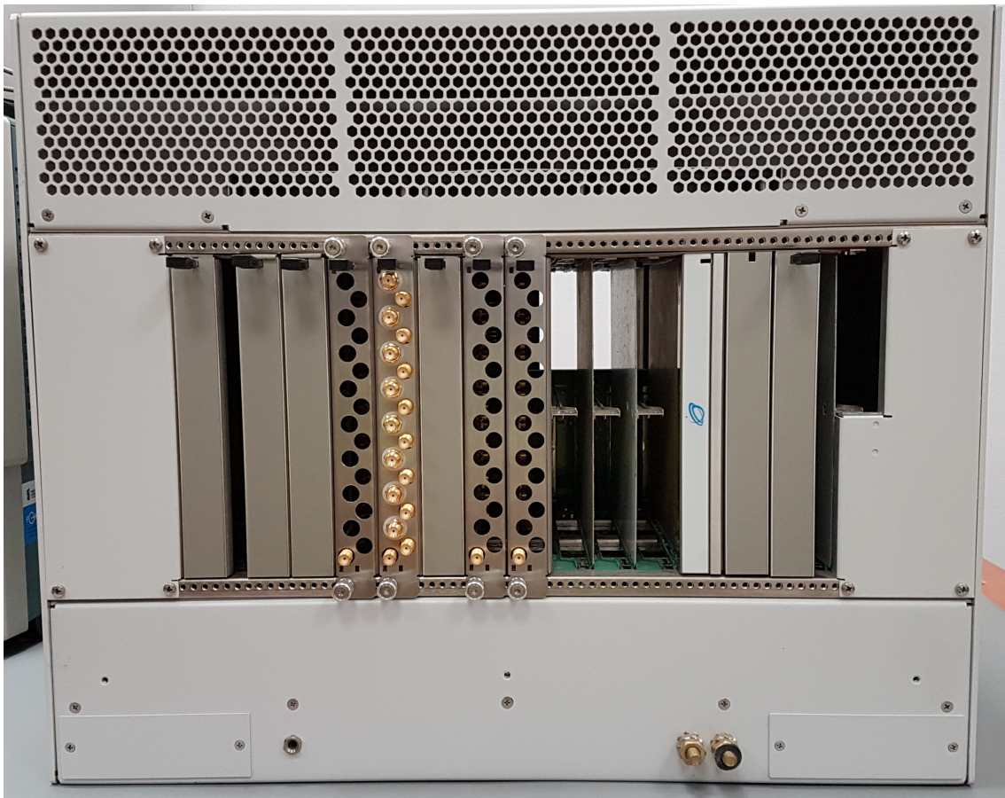
Figure 2: Micro TCA chassis with 4 RTM modules inserted. One of them has 4 BaseMod AFE mezzanines installed.
